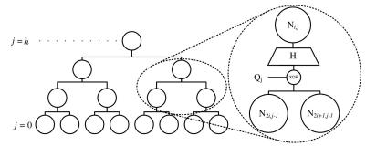
Fig. 1: The binary hash tree construction
