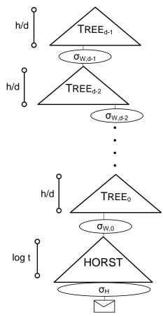
Fig. 3: Virtual structure of a SPHINCS signature
